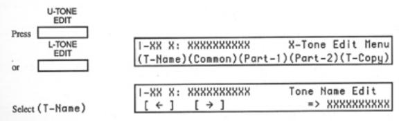
Move the blinking cursor with the KEY MODE and SPLIT POINT buttons; enter characters with the ten-key pad, the joystick, or the INCREMENT and DECREMENT buttons.
