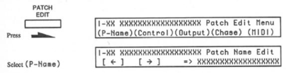
Move the blinking cursor with the KEY MODE and SPLIT POINT buttons; enter characters with the ten-key pad, the joystick, or the INCREMENT and DECREMENT buttons.
